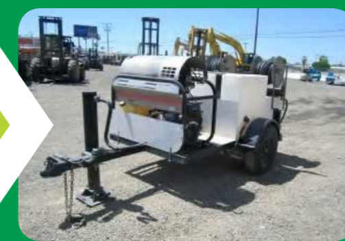
Trailer mounted Furphy pump systems and water carts are used to mitigate dust.
